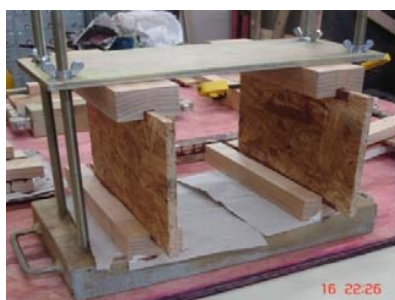
Fig. 5 Specimens on pressing apparatus
