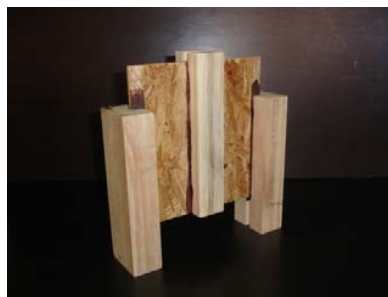
Fig. 6 Web-to-flange joint specimen with reinforcement
