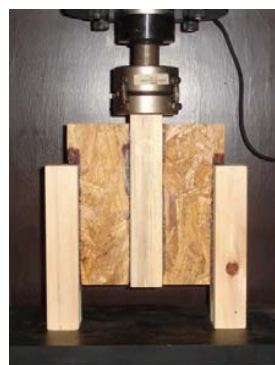
Fig. 7 Specimen in shear test machine
