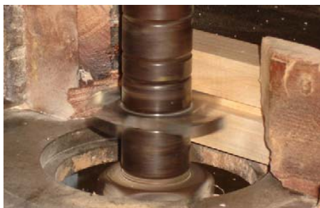
Fig. 4 Mortising machine producing the rectangular groove
