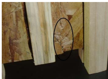
Fig. 8 OSB tore in shear near application line
