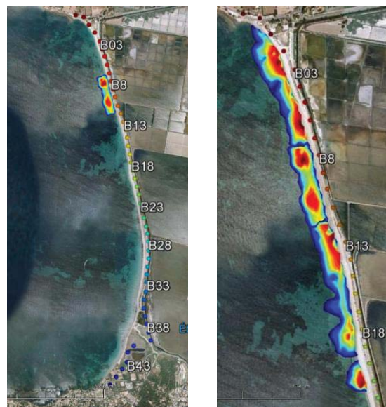
Fig. 2 Variation of bathymetry for alternative 1 - silting in the cell B (left) and alternative 2 - silting in the cells A to C (right).
