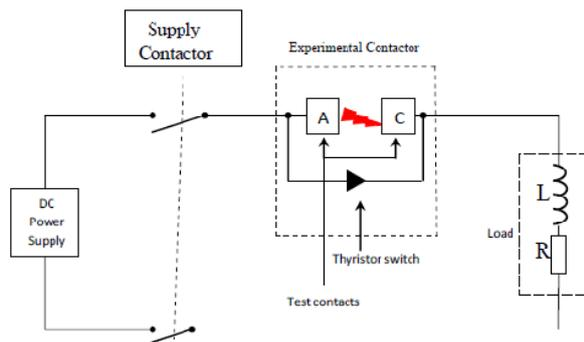
Fig. 4 Schematic diagram of the experimental contactor
