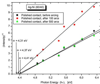
Fig. 8 Typical Fowler plots obtained by using (2) from EWF measurements for the polished Ag-Ni (60/40) contact, before arcing, and after 100 arcs and 500 arcs, in high vacuum  $1.4 \times 10^{-7}$  mbar
