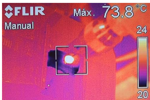
Fig. 8 Example of a thermography image without lubrication collected at the maximum temperature
