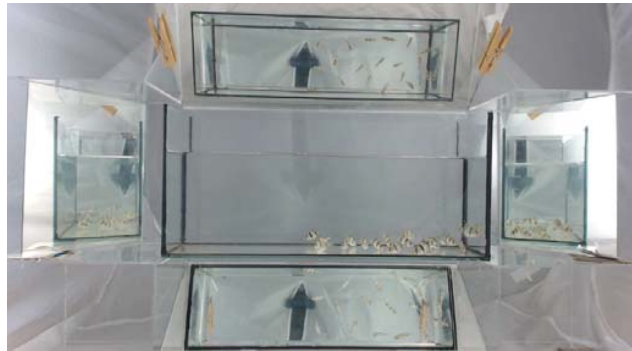
Fig. 1. The image of Puntius tetrazona shoal in the aquarium of the 5iD viewer. Construction of the system is clearly seen.
