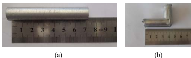
Fig. 2 Snap shots for sample (a) before and (b) after ECAP processing
