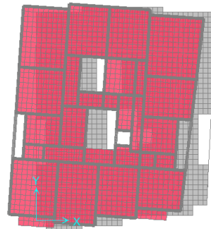
Fig. 10 (b) T_1=0.323 sec (Model II) infill wall
