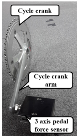
Fig. 1 Three-axis Pedal Force Measurement Sensor installed Device
