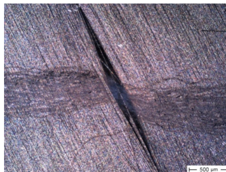
Fig. 1 Fish-Eye in a NCF in matrix made of carbon fibre; polyester binding yarn
