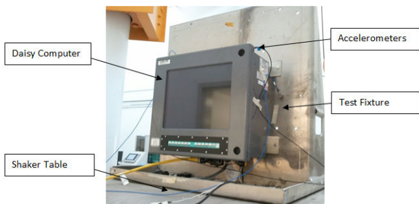
Fig. 3 Test setup for Daisy Data Displays computer
