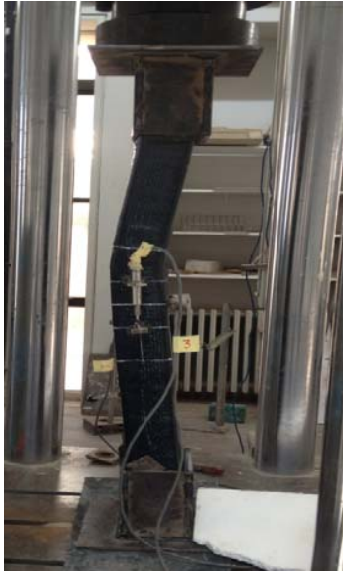
Fig. 4 Failure of CFRP wrapped specimen (NE)
