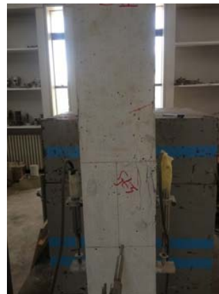
Fig. 3 Failure of control specimen
