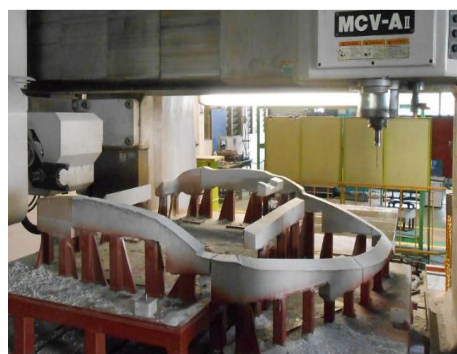
Fig. 1 Milling process for car door checking fixture
