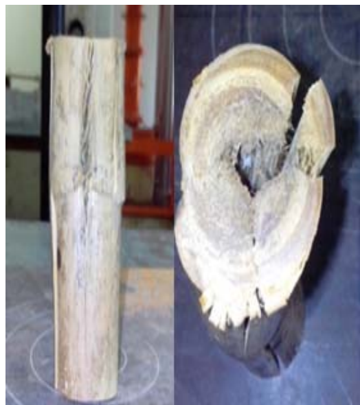
Fig. 3 Cracking and splitting mode of failure
