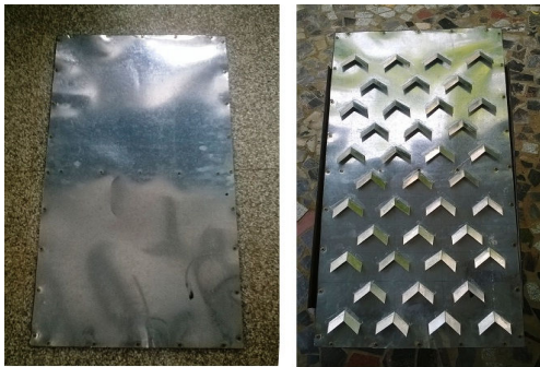
Fig. 3 Smooth and roughened absorber plate
