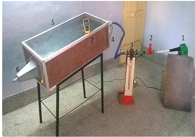
Fig. 2 Experimental setup of solar air collector system
