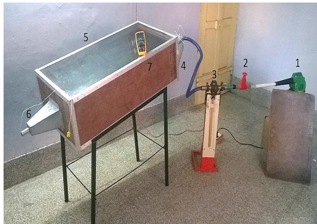
Fig. 2 Experimental setup of solar air collector system
