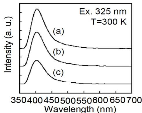
Fig. 3 PL spectra of Sr–Al–O:Eu<sup>2+</sup> phosphor particles at 300 K, (a) Sample 1, (b) Sample 2 and (c) Sample 3
