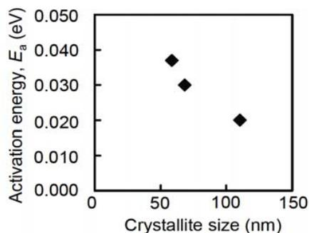
Fig. 7 Relationship between the activation energy and crystallite diameter size of Sr-Al-O:Eu<sup>2+</sup> phosphor particles
