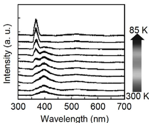
Fig. 4 CL spectra of Sample 1 at 85–300 K
