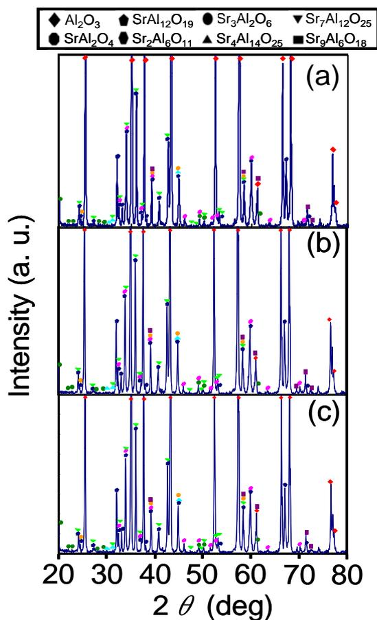
Fig. 2 XRD profiles of Sr–Al–O:Eu<sup>2+</sup> phosphor particles, (a) Sample 1, (b) Sample 2 and (c) Sample 3
