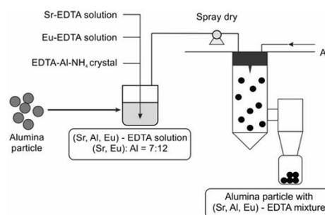
Fig. 1 Schematic diagram showing the preparation of a sample, including dispersion of alumina in the (Sr, Al, Eu)–EDTA solution made from Sr–EDTA solution, Eu–EDTA solution, and EDTA–Al–NH $_4$  crystals
