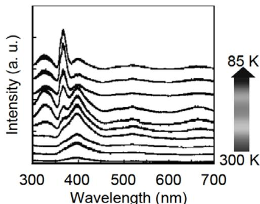
Fig. 6 CL spectra of Sample 3 at 85–300 K
