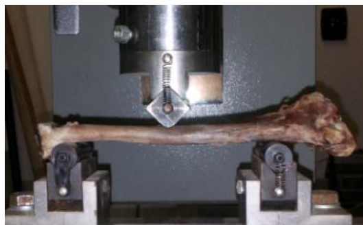
Fig. 2 Alignment of the specimen in three point bending measurement
