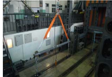
Fig. 7 Load test of single-beam hoist
