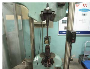
Fig. 6 Load test of the releasing device
