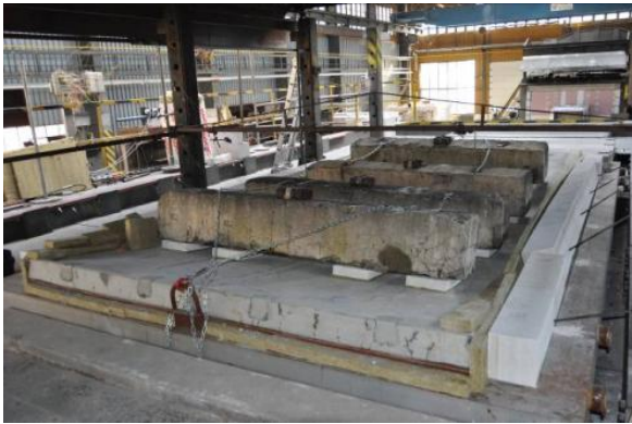
Fig. 1 Test slab after the 186 min of fire resistance testing
