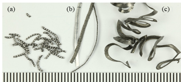
Fig. 7 Comparison of chip length of different titanium alloys: Ti-6Al-4V+0.9La (a), Ti-15Mo (b), and Ti-15Mo+0.8La (c)
