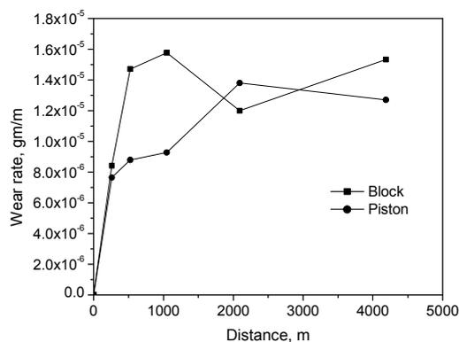
Fig. 4 Variation of wear rate (gm/m) with the variation of sliding distance (m) at applied pressure of 1.4 MPa (Load 20N) and sliding velocity 0.29 ms<sup>-1</sup>
