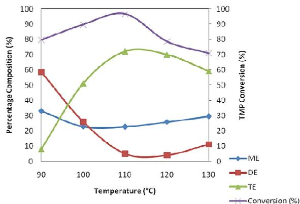
Fig. 6 Effect of temperature on the *Jatropha* oil conversion ( $p=50$  mbar, catalyst =3% w/w, TMP: JME=1:4,  $t=3$  h)
