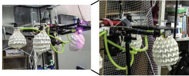
Fig. 8 Deflated Origami ball while the helicopter takes off and flies
