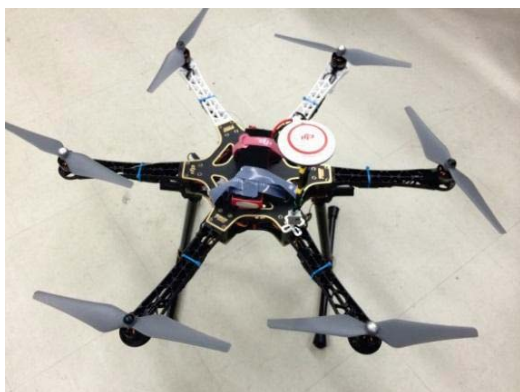
Fig. 1 Completely assembly of the DJI F550 Hexarotor
