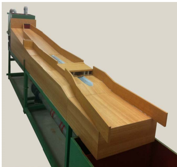
Fig. 2 Model of a storm water channel
