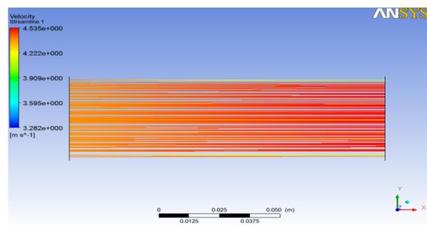
Fig. 6 Velocity streamline in 4 arc nozzle
