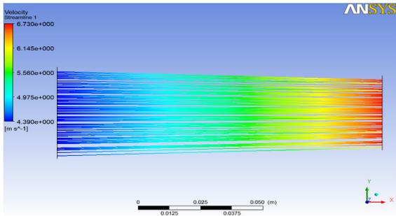
Fig. 7 Velocity streamline in 3 arc nozzle
