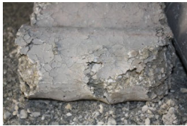
Fig. 6 Decomposition of a specimen exposed to 900°C
