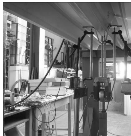
Fig. 4 Measuring instruments to vertical deflection
