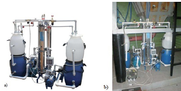
Fig. 12 Membrane pilot plant for wastewater treatment and concentrate utilization: a) 300 liter per hour membrane pilot plant; b) pilot testing at municipal wastewater facilities
