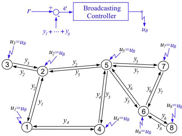
Fig. 1. Broadcasting Control of a Multi-agent System
