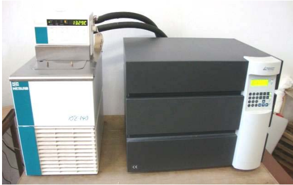
Fig. 3 Apparatus Holometrix 2300 for determination of thermal conductivity
