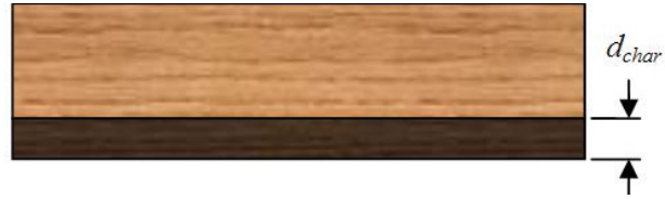
Fig. 2 Charring of timber – one dimensional
