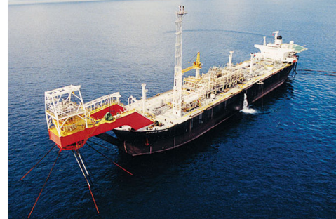
Fig. 1 Example of floating structure: FPSO [1]
