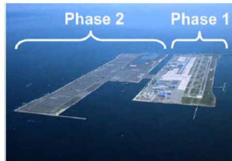
Fig. 2 Example of floating structure: Airport [2]
