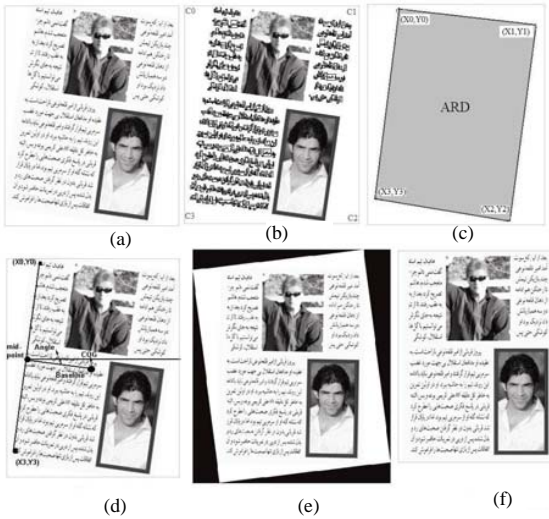
Fig. 1 (a) Skewed document image, (b) Document segmented to connected component, (c) The ARD in skewed document, (d) calculate the amount of document skew angle, (e) deskewed document, (f) final result
