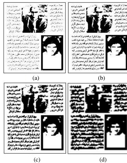
Fig. 4 Multi-scale images: (a) level 0 (480x670), (b) level 1 (240x335), (c) level 2 (120x167), and (d) level 3 (60x84)
