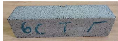
Fig. 9 PAG-10V specimen after 28 days of storing in CA solution
