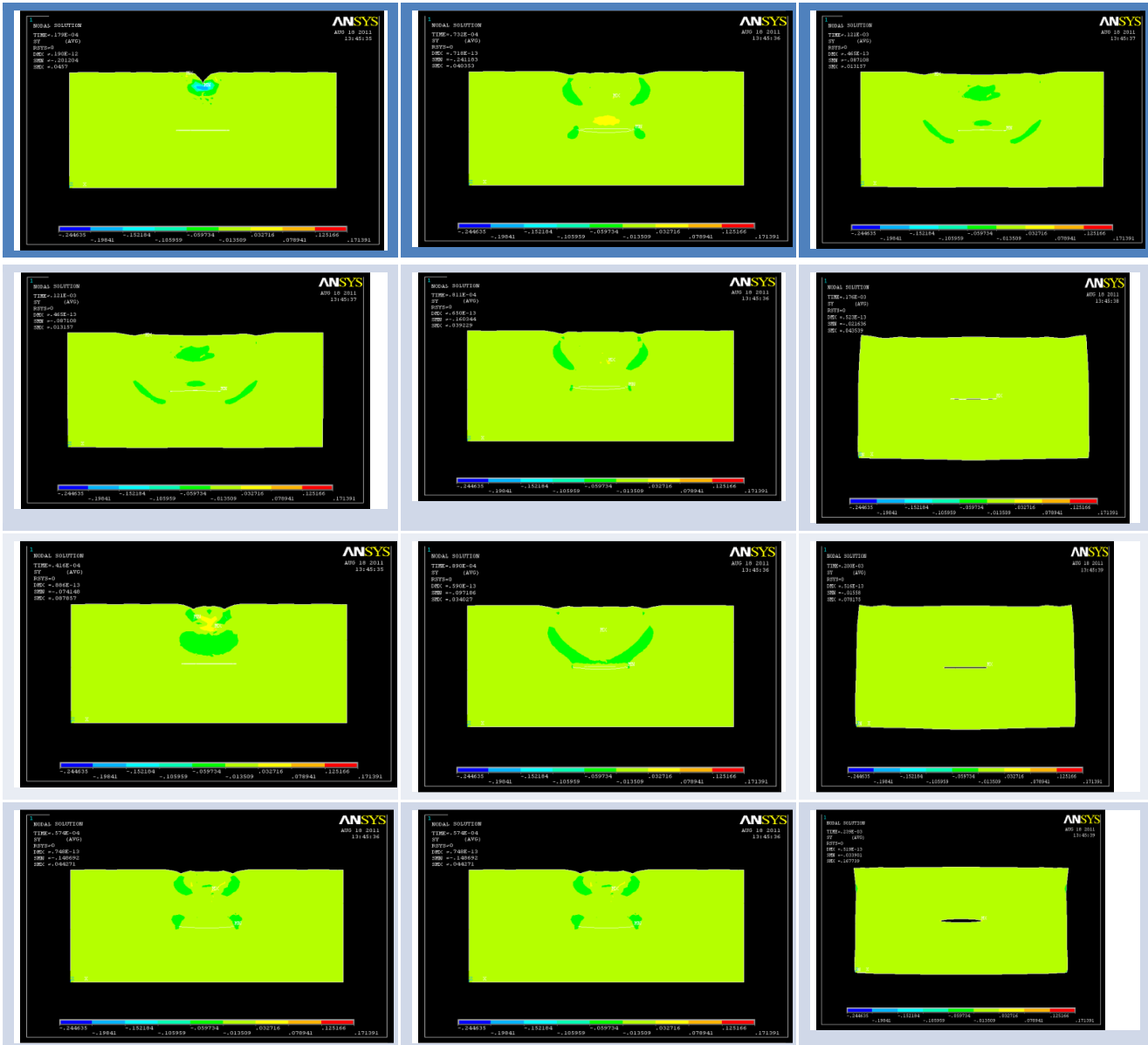
Fig. 20 Finite element simulation of impact on a plate, from top left to down, series of diagrams of shear wave
