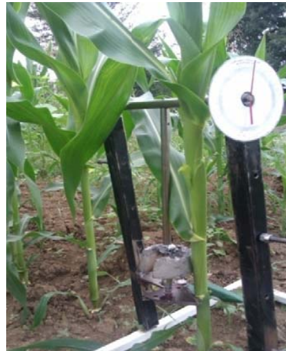
Fig. 2 Blade and finger statue during impact cutting
