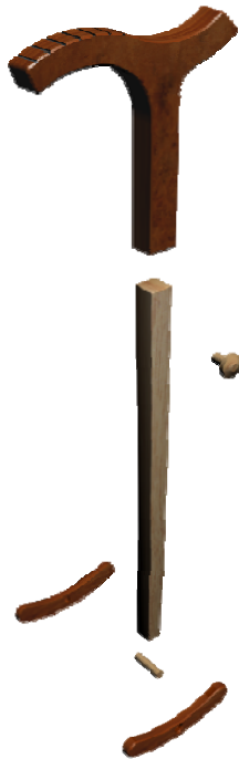
Fig. 5 Assembly of the walking stick for the Elderly
