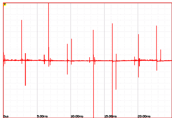
Fig. 15 Electrostatic discharges from the machine shaft
