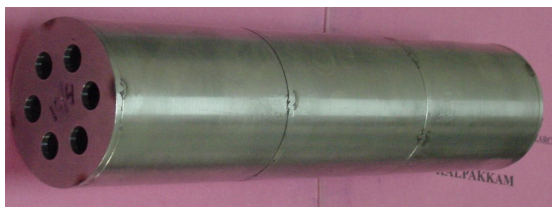
Fig. 11 Orifice assembly for blanket zone (Typical)
