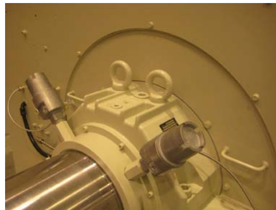
Fig. 6 Typical Bently Nevada connections are located with 45° [4]
