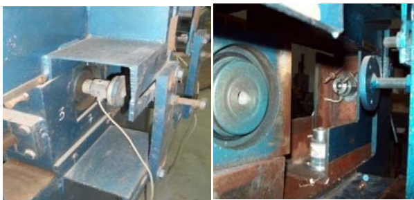
Fig. 7 Load cells attached with the roller bearings
