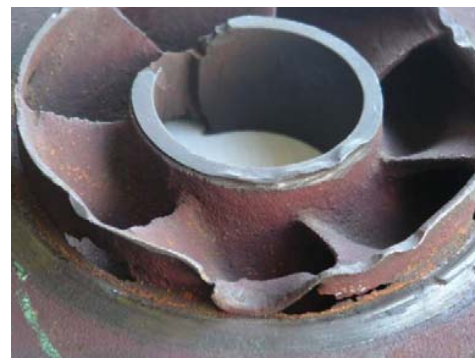
Fig. 3 The effects of cavitation in a sea water centrifugal lift pump impeller
