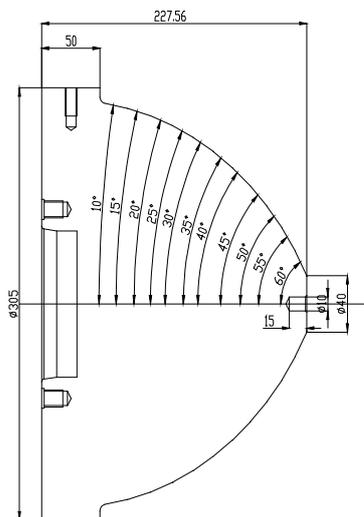
Fig. 1 Design of the formed parts used
