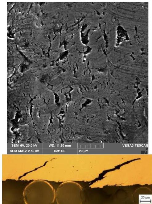
Fig. 6 Examples of the microcracks occurring in the surface of the sheet after forming using regular spinning parameters (Ti-Gr5 alloy) – SEM micrograph (top) and light microscopy (cross-section, unetched, 500 $\times$  magn.)
