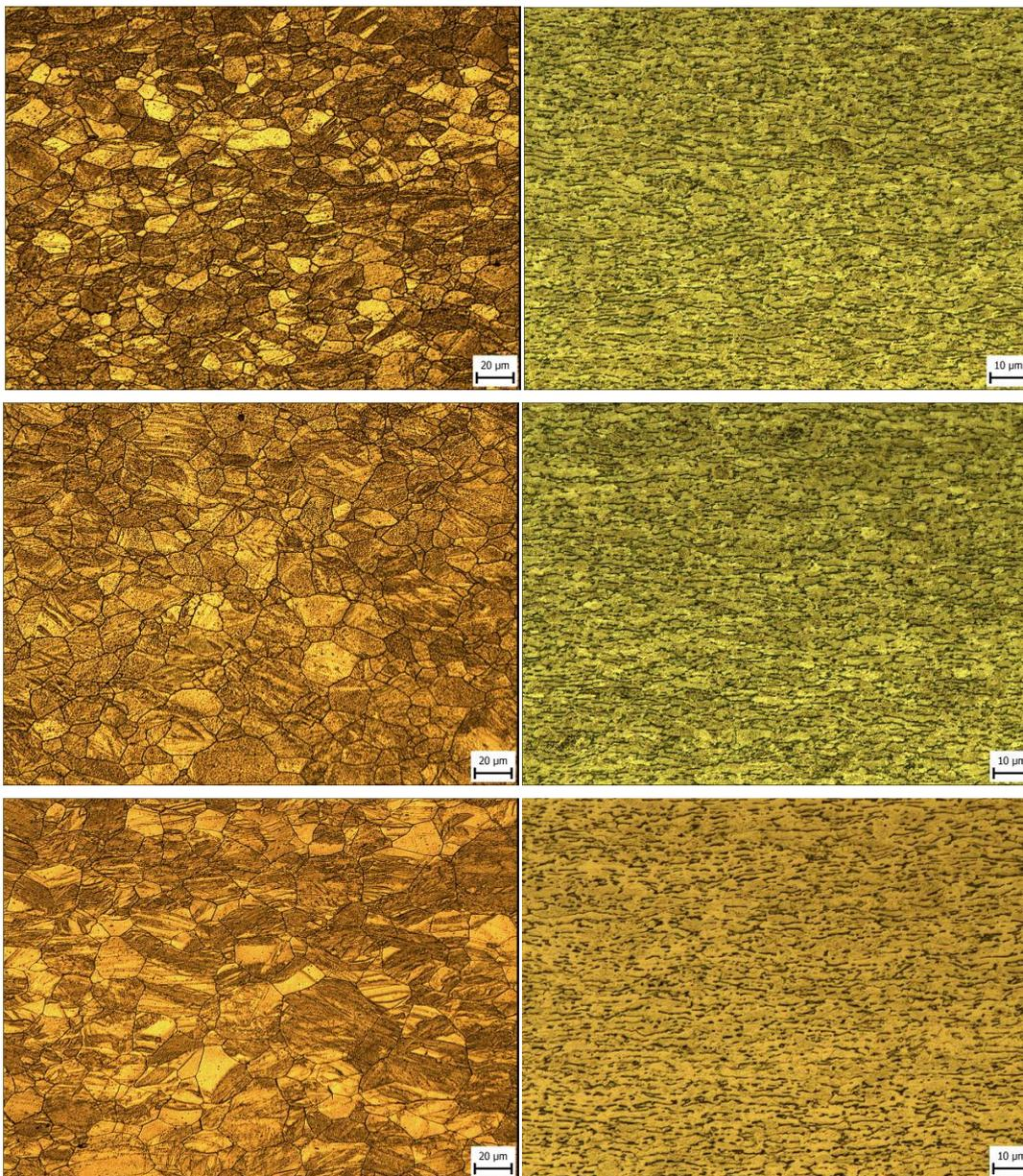
Fig. 3 Microstructure of the specimens taken from the CP titanium (left) and Ti-Gr5 alloy (right) deformed parts at wall angle of  $45^\circ$  – spinning mode (top), AISF mode (middle) and AISF parameters forming at spinning rates (bottom). Etched by the Kroll's and/or Weck's reagent. Magnification of  $500\times$  (left) and  $1000\times$  (right)
