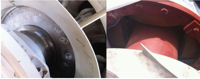
Fig. 29 Balancing weights positions (dynamic balancing panel-panel 2)
