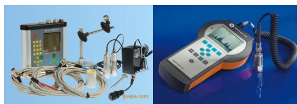
Fig. 2 Typical data collector with their side facilities like piezoelectric transducers (left easy viber and right vibro 60)
