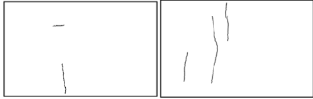
Fig. 8 Plastic shrinkage cracking 0.50% RP fiber, length 20mm
