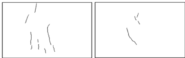
Fig. 10 Plastic shrinkage cracking 1.50% RP fiber, length 20mm
