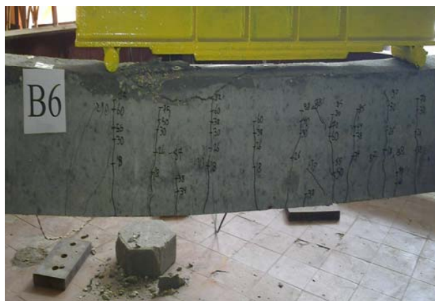
Fig. 7 Typical flexure failure for beam specimens
