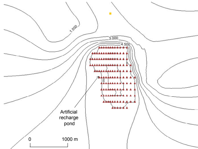
Fig. 10 Close-up of piezometric head around the recharge pond in layer 2 (0.5 m interval of contour line)
