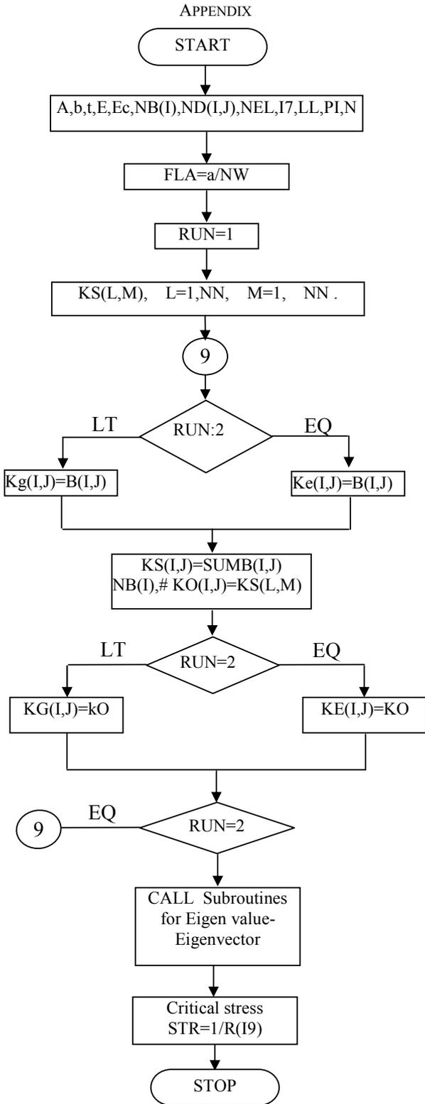
Fig. 7 Flow chart of plate buckling program
