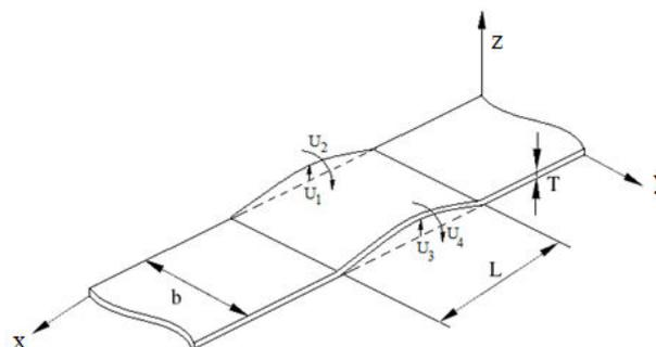
Fig. 1 Typical finite strip with nodal displacements
