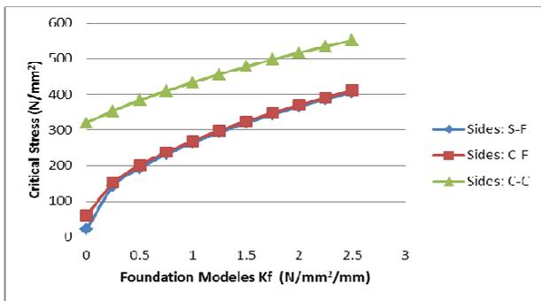
Fig. 4 Critical buckling stress for plates on foundation
