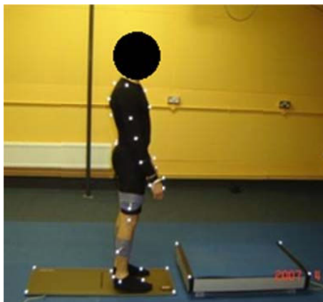
Fig. 1 The location of markers on the participant's body, following the 39-marker plug-in-gait protocol
