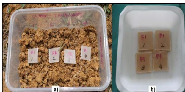
Fig. 7 Sample of LDPE/TS: 70/30 a) before and b) after the soil burial test
