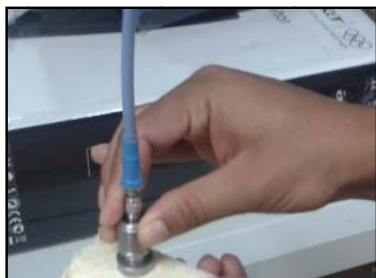
Fig. 3 Defining dielectric properties using dielectric probe
